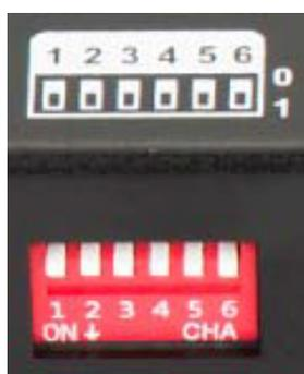
It is a 6 Bit binary switch, when the pin is pull up, its value is "0" ; when pull down, its value is '1". Its default setting is "000000" when you firstly received the units, we mark as group 00 in order to remember easily.
